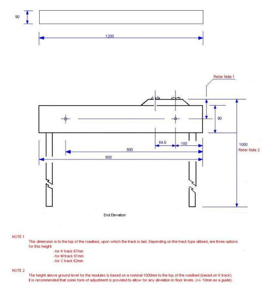
Please also note that the 1000mm the the top of the roadbed is based on K track, and some adjustment of this dimension may be required if an individual is using C or M track.
